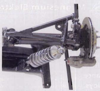
An example of Arning's four-link IRS with built-in steer action
